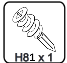
Wall Anchor (attaches to wall - not needed if screwing part H80 into a stud)
